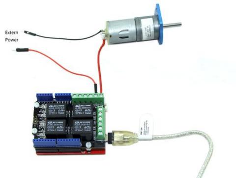
**Note:** We use a lithium battery as the power supply for the motor. Users can select other power sources as well. Of course, a power adapter will be essential when using high-current devices. 3. Restart the Arduino IDE. Copy the following code.
